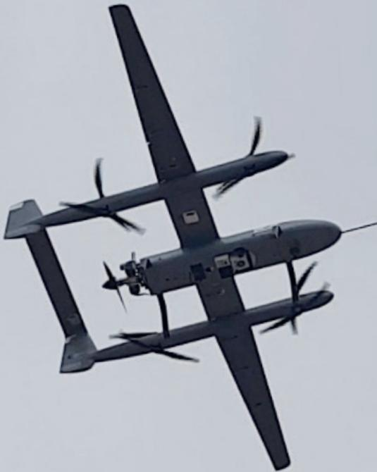
The **Laser Monitoring Fixed Wing (LMF)** is a sensor which is used for remote detection of methane utilizing a laser beam and is installed on an unmanned aerial vehicle (UAV).
